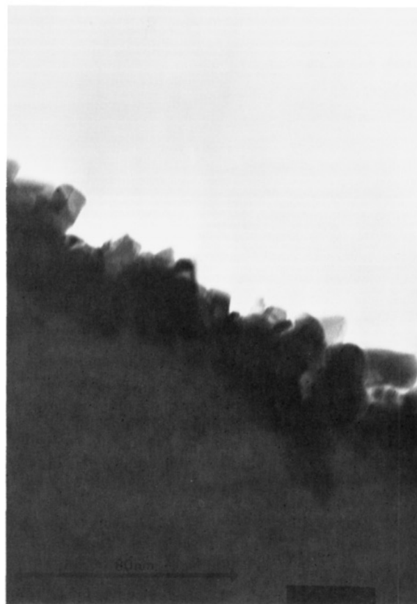
Figure 7. Transmission electron cross section of the surface region of a wet-air-cured 2 \times -doped BTDA-ODA film.
